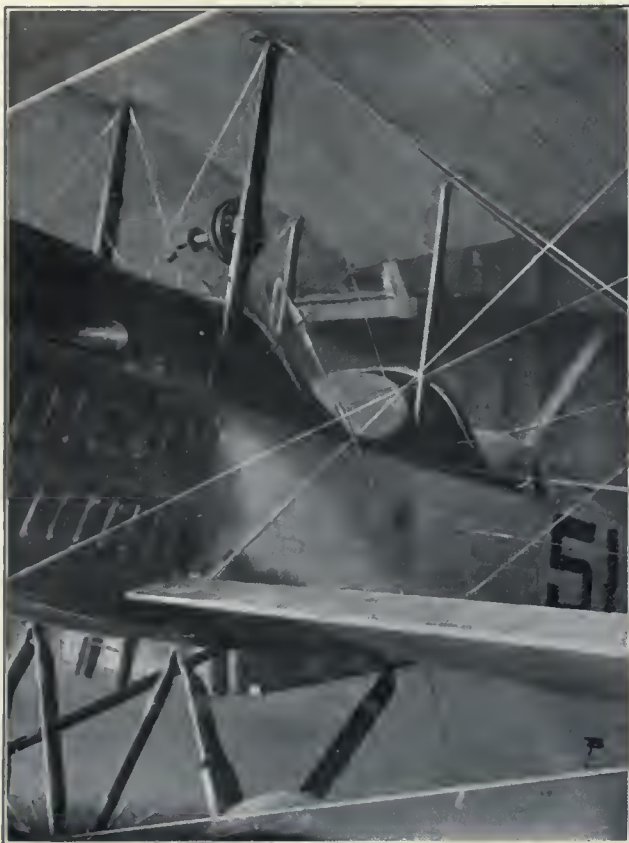
The reel and long copper tube of the Culver set through which the trailing aerial is paid out. This reel has now been replaced by one carried in the cock-pit.
