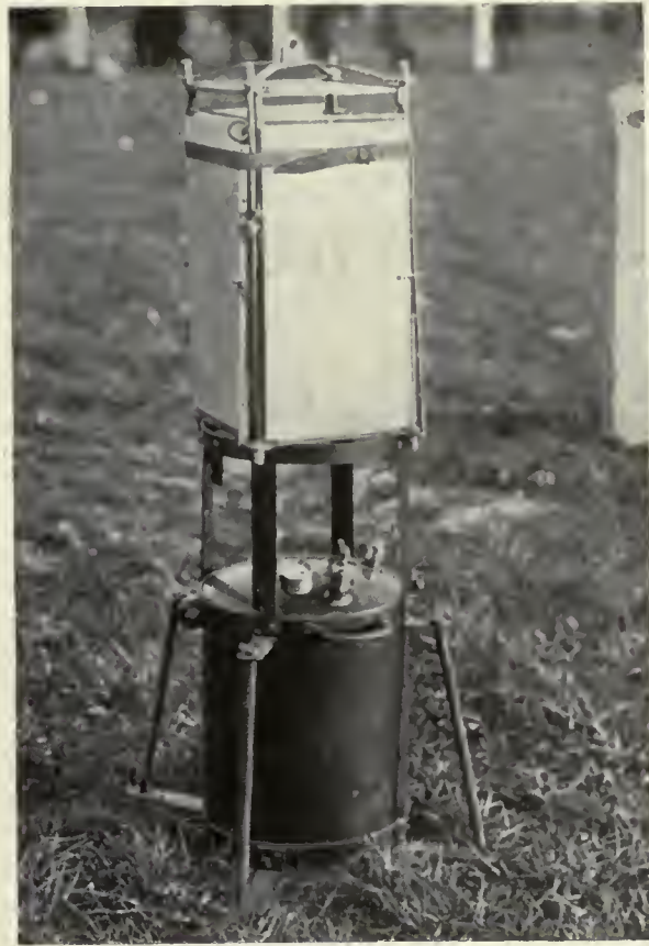
Portable aerial beacon of 2400 decimal C.P.
