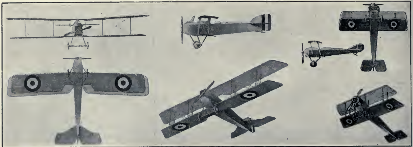
Bristol Scout (British). Called the "bullet." One of the fastest scouts. Uses a rotary Rhone engine. There is also a Bristol two-seater which has two pairs of struts at either side of the body. The two-seater is equipped with a fixed engine.
