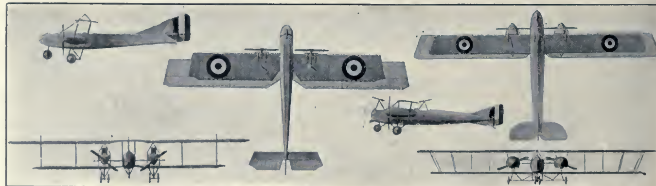
Letord. (French.) A three-plane twin-motored biplane tractor using fixed engines. The planes are staggered backward and the struts are run vertically backward at the tops.
