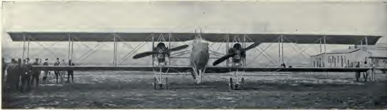
French Caudron biplane equipped with two motors. (Official French photo.)
