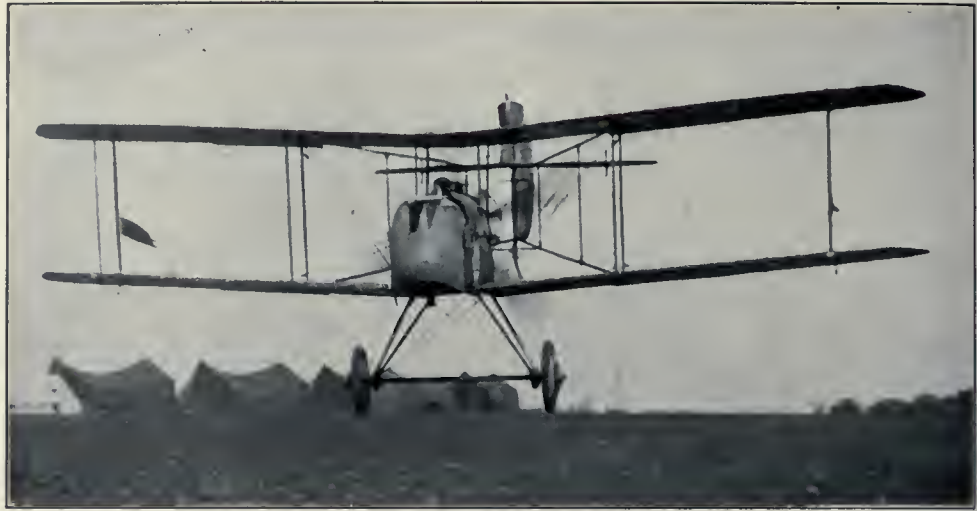
The DeHaviland Scout Bi-plane, one of the more recent British pusher-type scouts.
