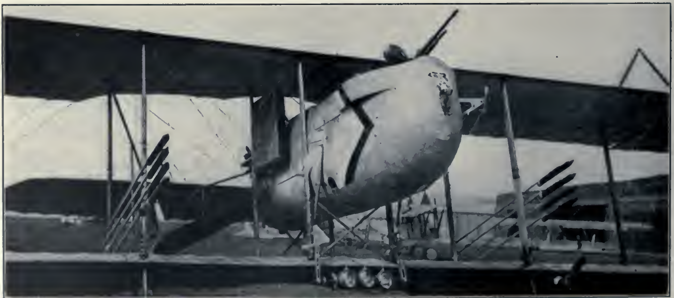
An Allied Zeppelin chaser which carries a machine gun mounted in front of the car, and attached to the frame work are a series of rockets, and below the lower wings a battery of searchlights. Note the rockets for setting Zeppelins on fire.
