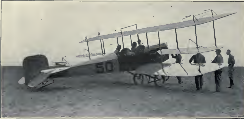
U. S. Army biplane used in Capt. Culver's experiments, showing radio apparatus and aerials.
