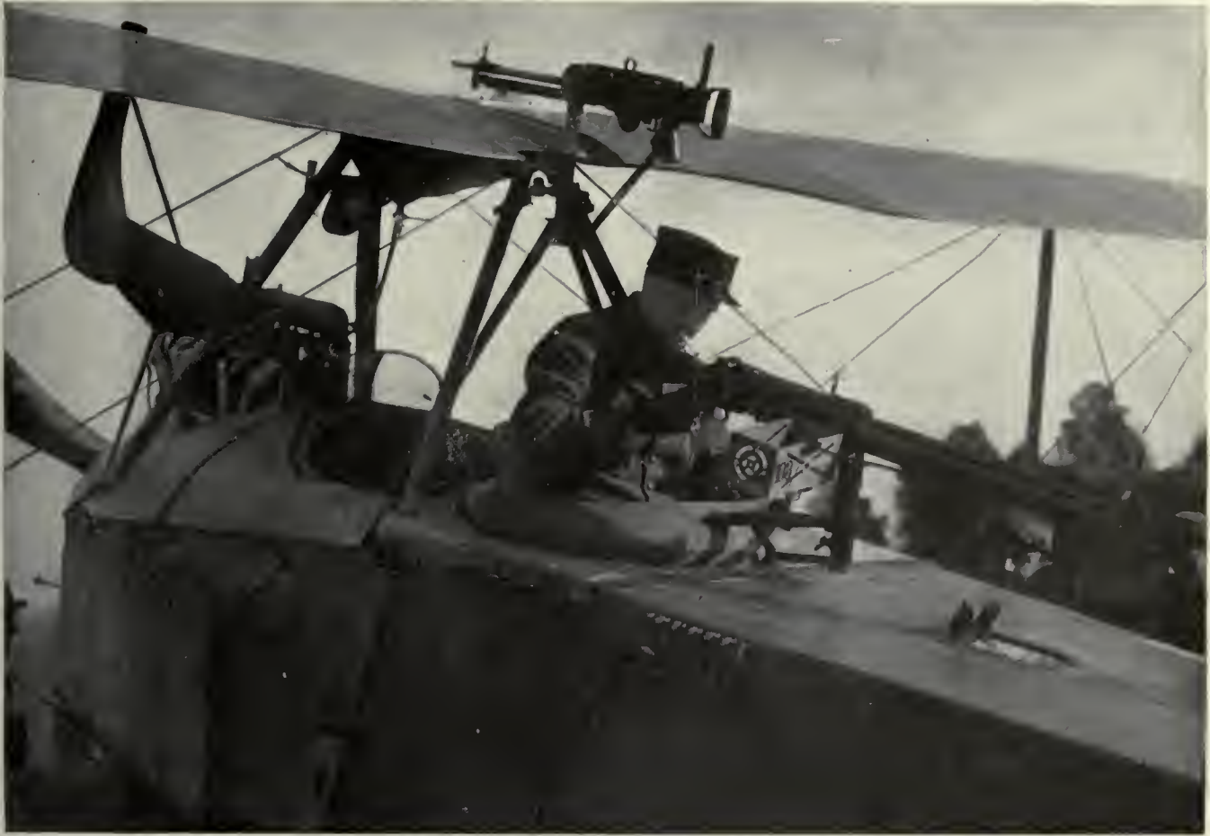
The famous French aviator Védrières examining the two guns of a German battleplane, which are so mounted that they can be shot in a half circle and up and down—through the hole in the fuselage.
