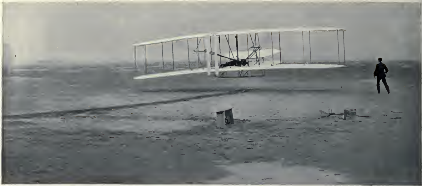
The first flight, December 17, 1903, Orville Wright at the helm; Wilber Wright alongside of machine. Date, December 17, 1903. Time, 10:30 a. m., 12:00 m. First flight, twelve seconds. Longest flight, fifty-nine seconds. Wind velocity, twenty to twenty-five miles per hour. Weight of machine, 605 pounds. Total weight, with operator, 750 pounds. Power of motor, ten to twelve horsepower. Weight carried per horsepower, sixty-three pounds. Speed of motor in flight, 1020 r.p.m. Speed of propeller, 310 r.p.m. Spread of wings, forty feet, four inches. Length of chord, six feet, six inches. Total area of wings, 530 square feet. Area of elevator forty-eight square feet. Area of vertical rudder, twenty square feet.
