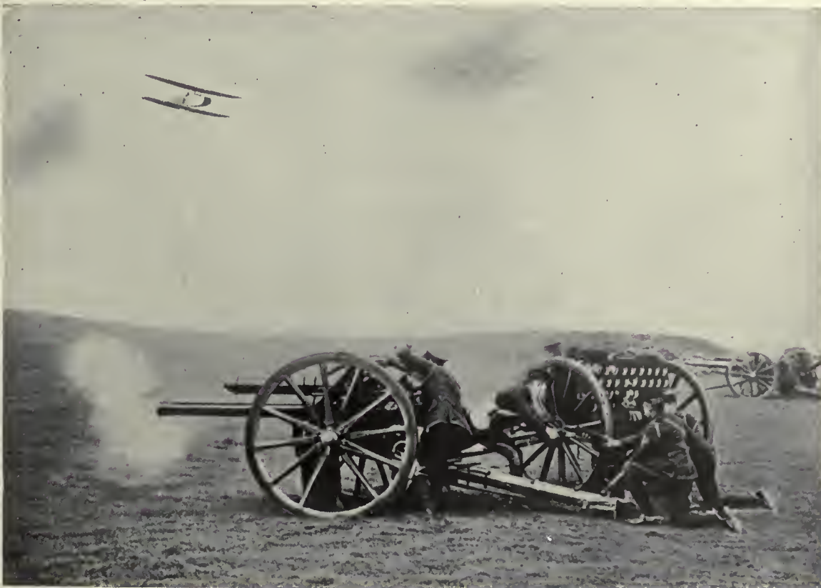
An aeroplane being used for artillery fire. The aeroplane circles over the firing batteries and the observer watches the effect of the shots and directs the man behind the guns by wireless.
