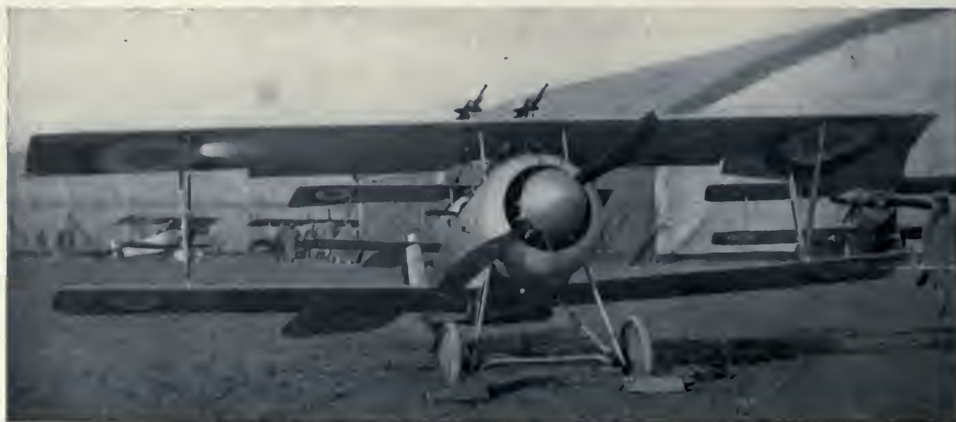
The 1917 type Nieuport avion de chasse, equipped with two Lewis guns shooting over the planes, and a Vickers gun to shoot through the propeller. In the rear can be seen a "Spad" and several Nieuports.
