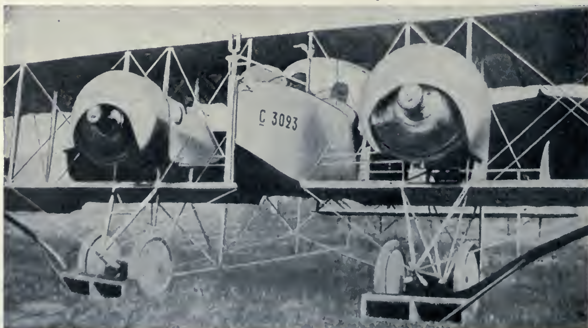
A "G-4" Caudron biplane, equipped with two 80 h.p. Le Rhone motors. The gun mounting is seen in front.
