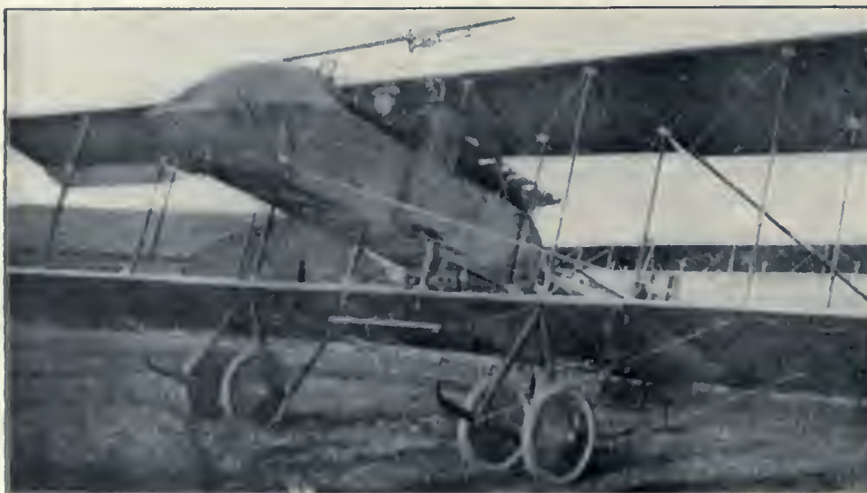
A Davis non-recoil gun mounted on a British battleplane. The three inch gun of this type shoots a 15 pounder.
