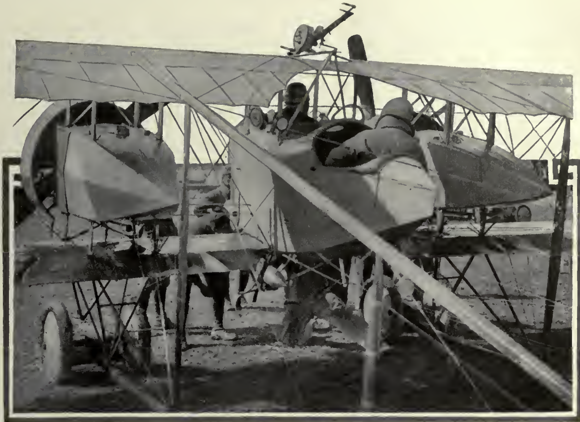
A double-motored Caudron biplane used extensively for observation, in France. It is equipped with a Lewis gun.
