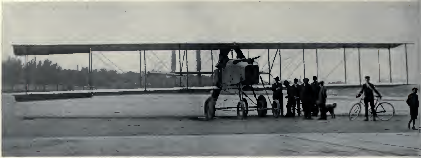
The first "gun-plane" was the French Voisin armored and armed with a 37 mill. gun, tested early in 1914. It disproved the theory that the recoil of a gun would upset the aeroplane.
