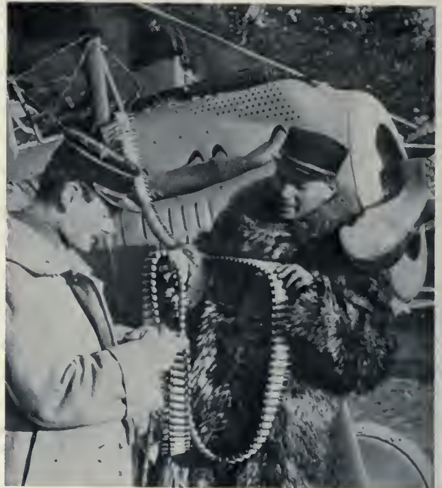
A Vickers gun mounted on the "Spad" of a member of the Lafayette Flying Corps, and the belt with which it is fed.
