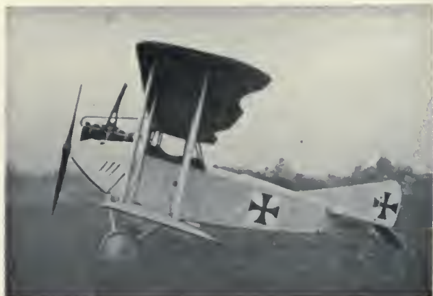
The A. E. G. 1917 single motored type of German biplane, equipped with a 175 h.p. Mercedes motor.
